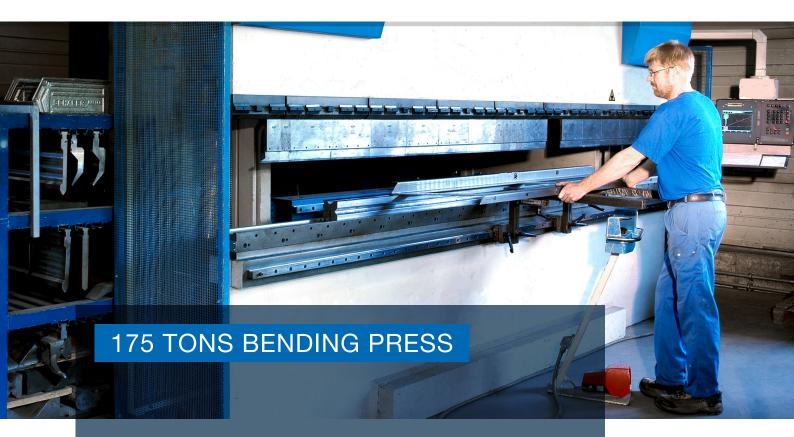
In the field of sheet metal forming, Leiritz uses the 175-ton bending press to perform precise series bending sheet metal processing and to further process it into various sheet metal welded constructions.
