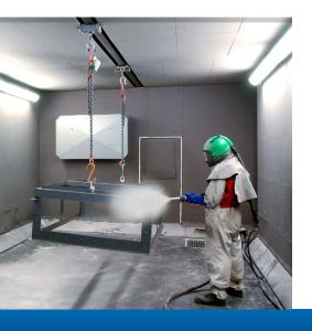
In the company's own painting hall (13.5 x 4 x 3.5 metres), all common painting systems and special paints are processed using the latest painting technology with airless system incl. E-static and 2K mixing unit. Thus, the mechanical engineering parts and plants are coated cost-effectively and, above all, in an environmentally friendly manner.
